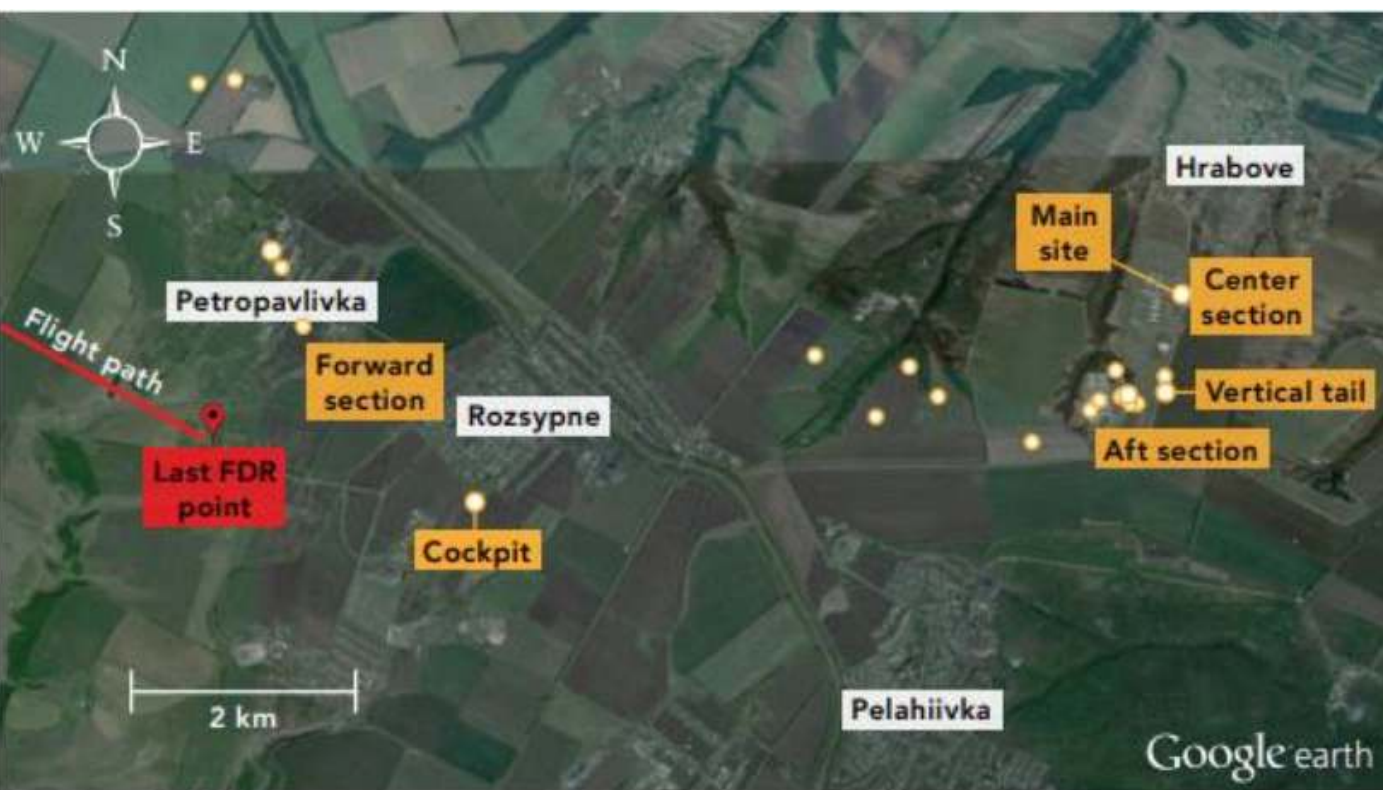
Figure 6: The last location of the aircraft in flight taken from the FDR. Wreckage distribution is grouped per section of the aircraft (Source: Google Earth, wreckage information Dutch Safety Board).
