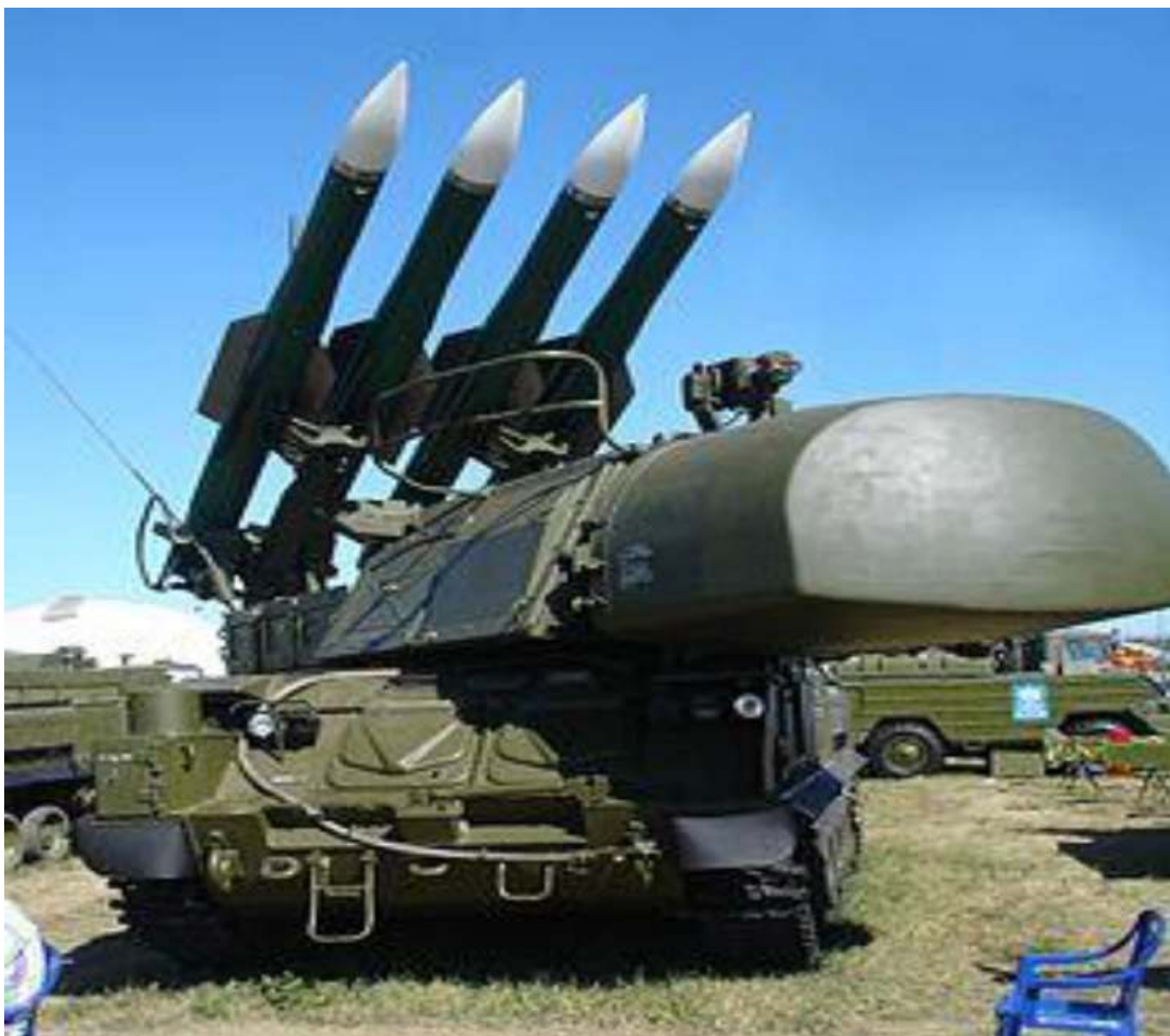
واحد بوک-تیلار (Transporter Erector Launcher and Radar).
